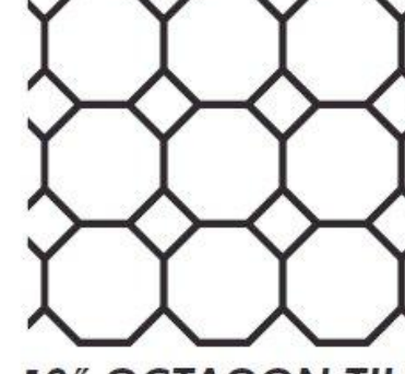
10" OCTAGON TILE OCTAGON DIAMETER: 10 1/4" ROLL WIDTH: 33 1/2" JOINT WIDTH: 11/16"
