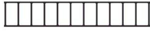
BRICK HEADER BRICK SIZE: 3 \frac{7}{8}'' \times 7 \frac{7}{8}'' ROLL WIDTH: 8 \frac{3}{4}'' JOINT WIDTH: \frac{1}{2}''
