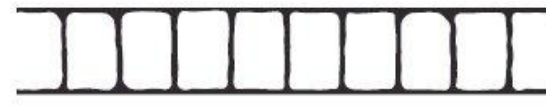
COBBLE HEADER BRICK SIZE: 4 \frac{3}{4}'' \times 7 \frac{1}{2}'' ROLL WIDTH: 8 \frac{3}{8}'' JOINT WIDTH: \frac{1}{2}''
