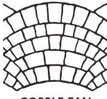
COBBLE FAN BRICK SIZE: RANDOM ROLL WIDTH: 34" JOINT WIDTH: 1/2" - 3/4"
