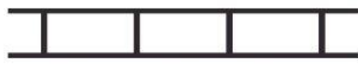
EDGE BRICK HEADER BRICK SIZE: 4 \frac{1}{8}'' \times 8 \frac{13}{16}'' ROLL WIDTH: 5 \frac{1}{8}'' JOINT WIDTH: \frac{1}{2}''
