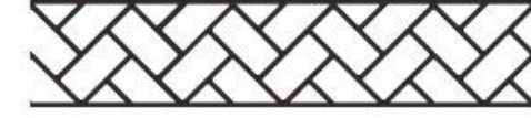
HERRINGBONE HEADER BRICK SIZE: 3 \frac{3}{8}'' \times 7 \frac{5}{16}'' ROLL WIDTH: 8 \frac{5}{16}'' JOINT WIDTH: \frac{1}{2}''
